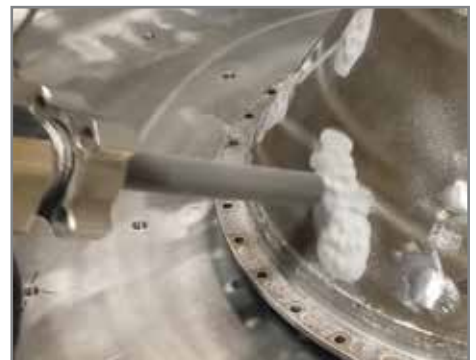
Accelerating powders at supersonic velocities to restore hard-to-find parts
