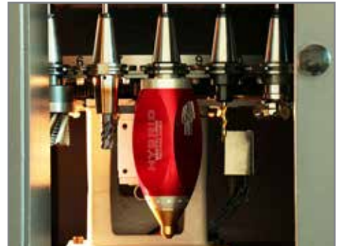
Combining additive and CNC (subtractive) technologies to make new parts and repairs
